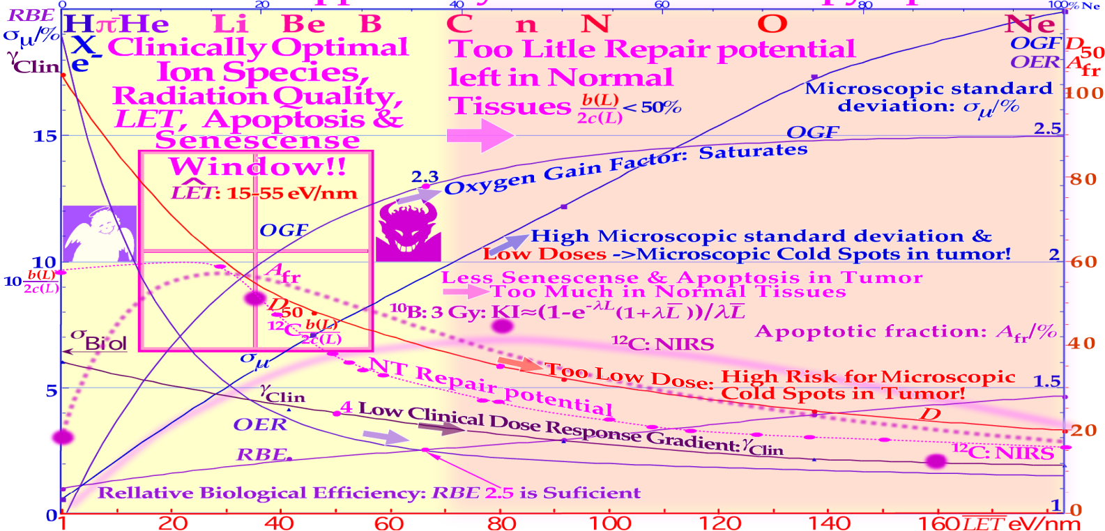
Figure 39: The LET variation of key biological parameters that influence the clinical value of radiation beams showing that the optimal window of opportunity in radiation therapy optimization is located between about 15 and 55 eV/nm or He-B ions. The underlying data are collected from Berkeley, NIRS and Karolinska. Interestingly, many of the above quantities can be biologically optimized by the methods discussed in [13]: Table 2 to ensure maximum complication free cure in the treatment! The rather low final dose increments in a high-LET and high-microscopic heterogeneity treatment will inevitably generate microscopic cold spots where some of the few remaining tumor clonogens may survive!
