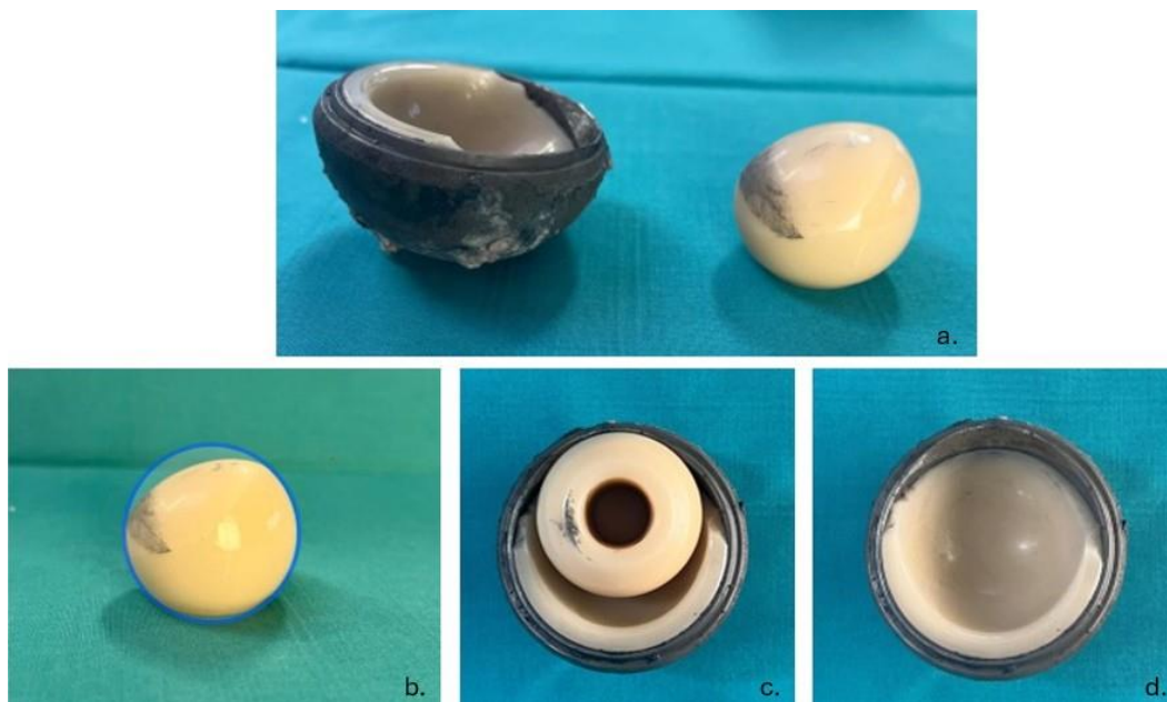
Figure 4. Retrieved worn implants (a)* Acetabular components and ceramic femoral head ; (b)* Wear and loss of sphericity of the ceramic femoral head ; (c)* Ceramic femoral head in situ ; (d)* Wear of the ceramic liner with exposure of the metal-back
