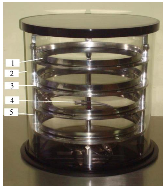
Figure Legend 2: Vacuum chamber of the Rificor L-A-B4-C Freeze dryer. 1. Tray; 2. Transparent vacuum chamber; 3. Temperature-controlled shelf. 4. Product temperature sensor; 5. Framework supporting the structure of the shelves under high vacuum.
