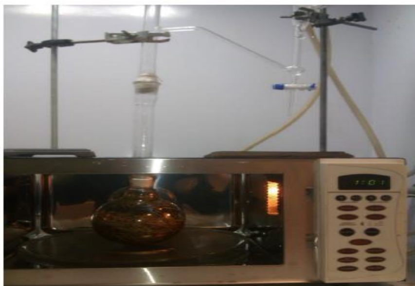
Figure 2.4. A Microwave assisted extraction set up (containing microwave, retort stands, condensers, and flat bottomed flask holding the samples under extraction).
