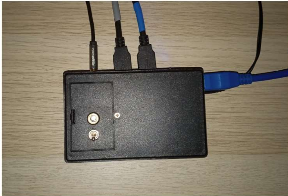
Figure 3: USB 3.0 hub to connect webcams to PC and driving top laser level
