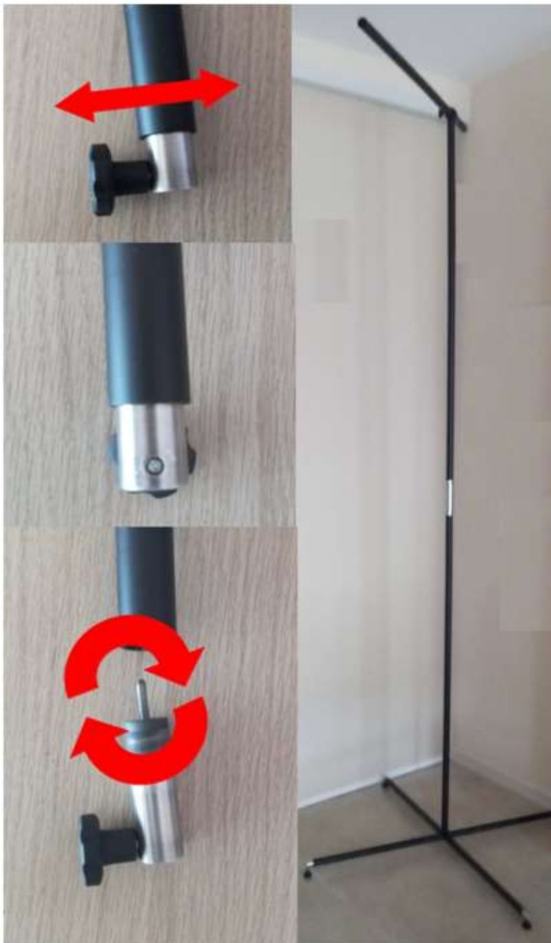
Figure 7: Outdoor support for top view webcam and details
