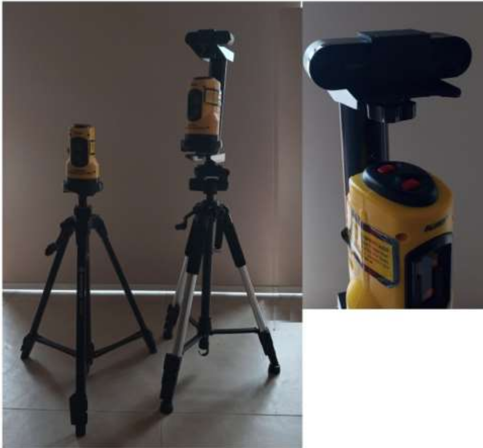
Figure 2: Tripod for supporting laser level and 4K webcam with detail
