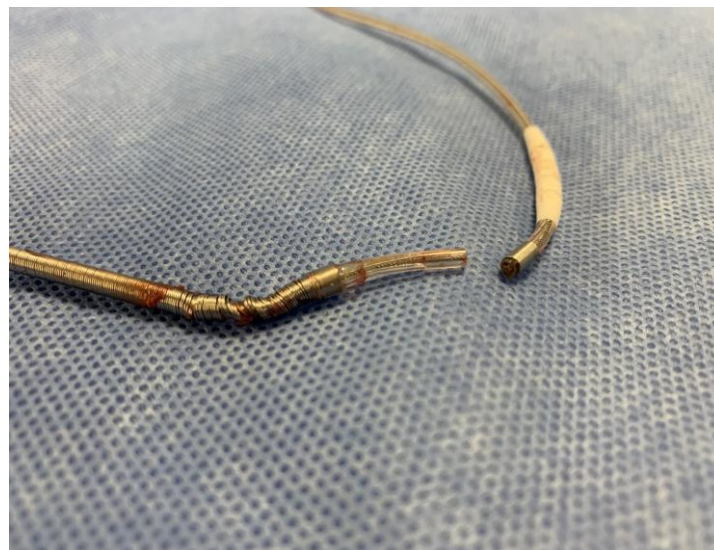
Figure 4: Emblem S-ICD lead fracture post explantation.
