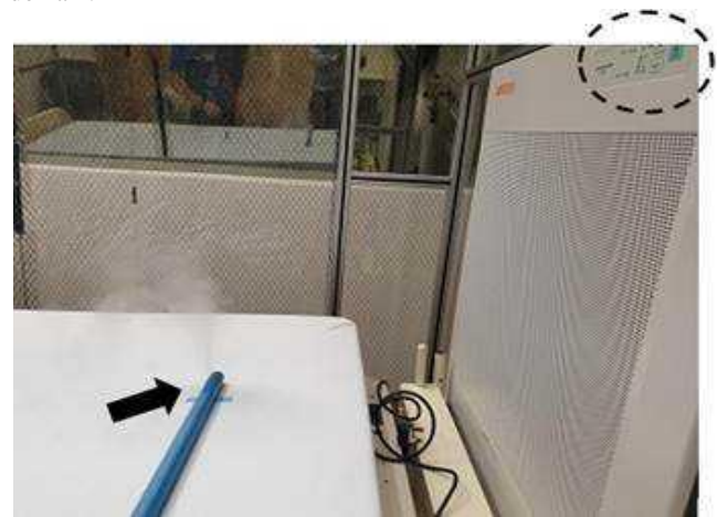
Fig 3: Introducing the “smoke”: When the HEPA filter is in the OFF mode (circle) the smoke lingers around the enclosure of the tent pressure with the NPFIT
